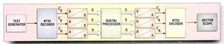
Figure 6. Test setup for measurements of hybrid equipment.
