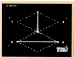
Figure 12. Diamond display of a legal signal.
