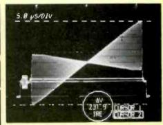
Figure 11. The encoded composite analog NTSC signal generated by the Y, B-Y, R-Y component analog ramps. Note the significant — and illegal — negative and positive exclusions.
