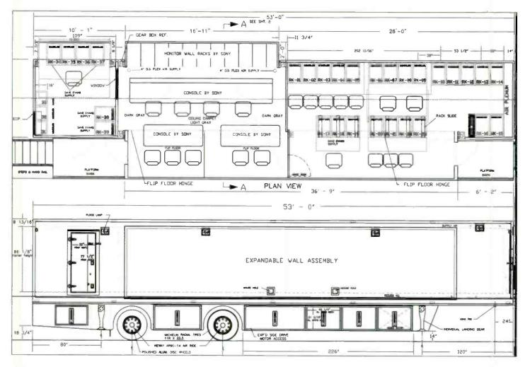
Note the expanding section shown above is primarily "people space" and adds about 180 square feet of working room. NMT's HD-1 will be the first digital high-definition truck to hit the road. The project was handled by Sony's Systems Integration Center.
