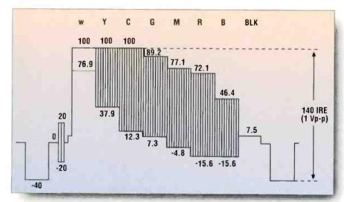
Figure 4. NTSC 75/7.5/75/7.5 color bars signal waveform.
