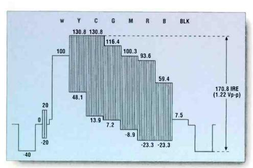
Figure 3. NTSC 100/7.5/100/7.5 color bars signal waveform.
