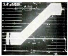
Figure 5. Modulated ramp test signal.
