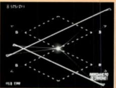
Figure 13. Diamond display of an illegal signal.
