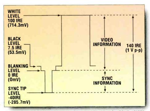
Figure 1. Significant amplitude values of a composite video signal in the 525/60 standard.
